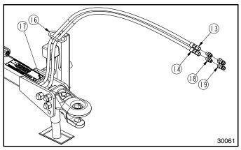
Hydraulic Hose Routing & Quick Coupling Assembly Figure 1-4
